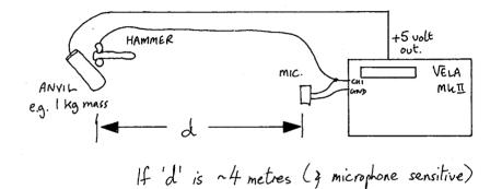
then velocity of sound in air may be measured with ~ 1% precision SET EXTERNAL/INTERNAL SWITCH TO INTERNAL, AND CH1 TO ± 250 mV.
