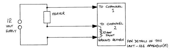
SET CH 1 INPUT TO  $\pm$  25V, CH 2 INPUT TO  $\pm$  250mV. USE A 10A SHUNT.
