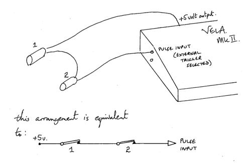
DO ENSURE THAT THE LIGHT BEAMS ARE CUT BY AN OPAQUE (SEWARE OF THIN CARD OR CARDBOARD !! ) MATERIAL AND THAT THE PHOTODIODES/PHOTO-TRANSISTORS ARE SHIELDED FROM UNWANTED LIGHT.
