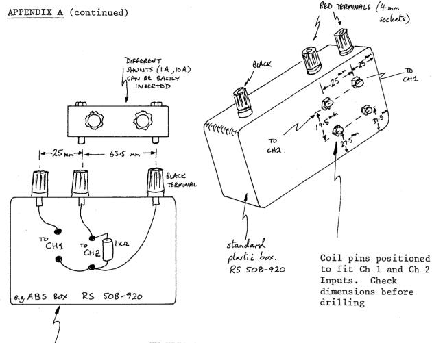
INTERNAL VIEW OF BOX. IN TRIALS THIS ARRANGEMENT MADE IT MUCH EASIER FOR STAFF AND PUPILS TO SIMPLY VIEW CH 2 AS A CURRENT RANGE. THE  $1k\Omega$  RESISTOR REPLACES THE 1000  $\Omega$  METER. THE BASIC BOX WITHOUT ADDITIONAL SHUNTS CORRES-PONDS TO A CURRENT OF 100  $\mu$ A. YOU ARE ADVISED TO AVOID USE OF DUAL RANGE SHUNTS, AS THESE CAN GIVE FALSE RESULTS BECAUSE OF THE COMMON NEGATIVE USED BY CH 1 AND CH 2 INPUTS.
