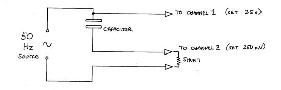
CHANNEL 1 MEASURES VOLTAGE, CH2 MEASURES CURRENT (SEE APPENDIX A). A SHUNT OF 1mA IS SUITABLE AND VELA INDICATES THE PHASE LAG OF CURRENT COMPARED TO VOLTAGE, i.e. 270 DEGREES (EQUIVALENT TO CURRENT LEADING VOLTAGE BY 90 DEGREES). USE OF A TWIN BEAM OSCILLOSCOPE PROVIDES VISUAL SUPPORT FOR THE MEASUREMENT.
