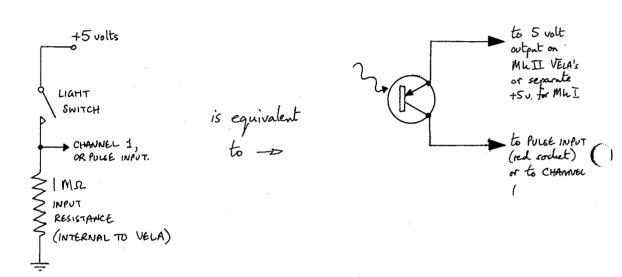
THIS WORKS RELIABLY FOR PHOTODIODE R.S. 305 - 462TAND I.R. DETECTOR R.S.  $306 - 083^{T}$  provided they ARE WELL SHIELDED FROM EXTRANEOUS LIGHT AND THAT THE CARD, etc. USED TO CUT THE LIGHT BEAM IS TRULY OPAQUE.
