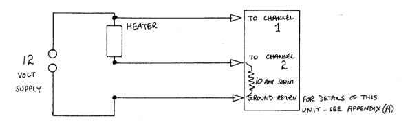
SET CH 1 INPUT TO  $\pm 25V$ , CH 2 INPUT TO  $\pm 250$  mV. USE A 10A SHUNT.
